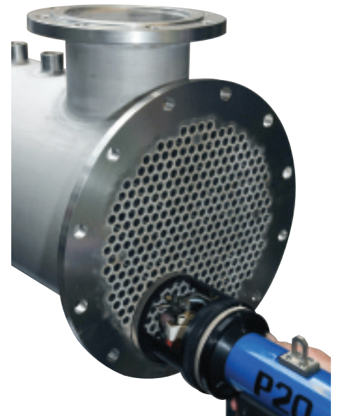
Automated tube end welding and 100% inspection
